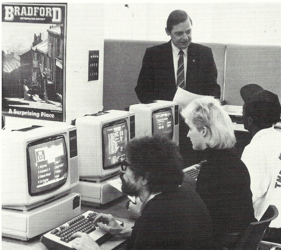
After shopping clerks at Centrepoint have taken orders from its elderly and disabled customers these are then entered into the system using videotex terminals. This information is then processed on a ROCC 2840 and forwarded to the relevant retailer where Centrepoint staff assemble the shopping orders for delivery, usually on the next day.
