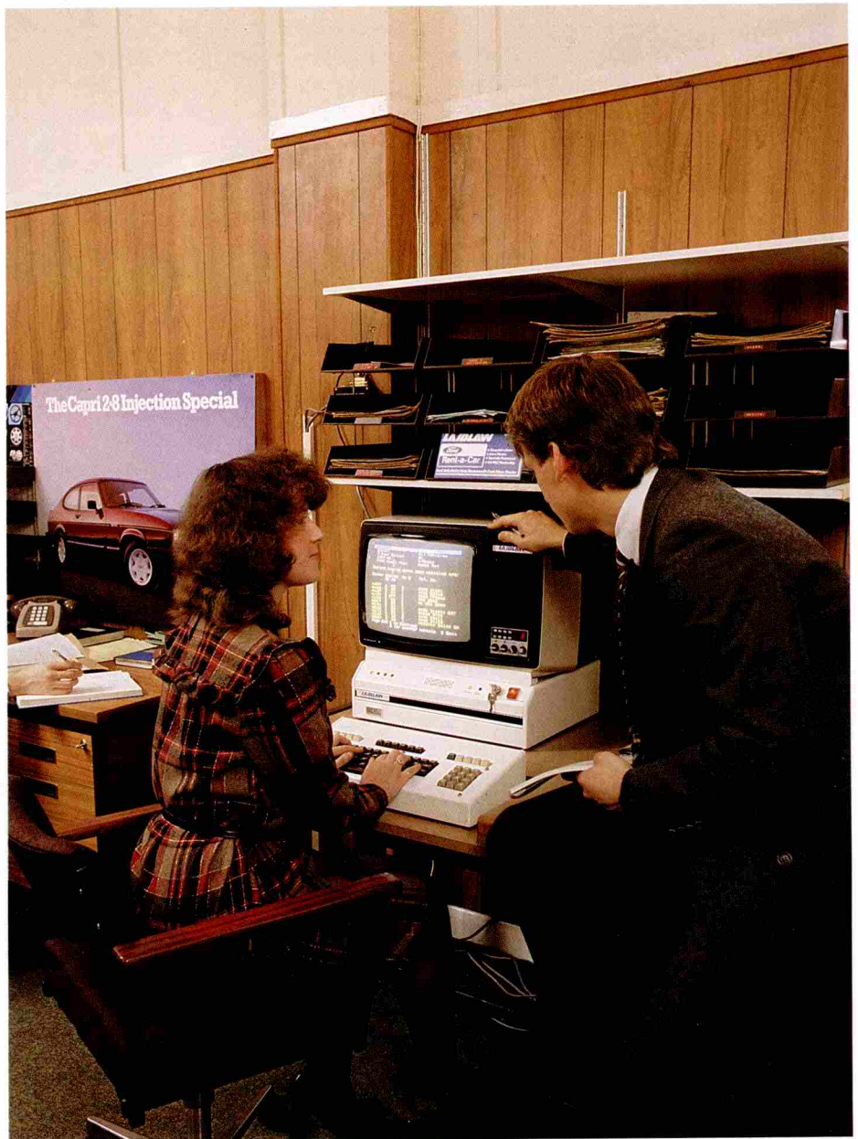
Picture shows Ford's viewdata vehicle locator system being used at Laidlaw, a Ford main dealer in Brentwood. The salesman is running through the customer's vehicle option specification to see where there is an identical vehicle available in the UK, so that Laidlaw can 'adopt' it.
